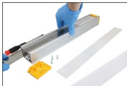
Insert the polarizer under the TR window
