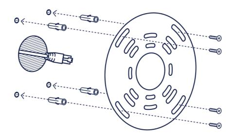
Mount bracket to the wall or ceiling with included mounting hardware. Thread the Ethernet cable and/or power adapter cable through the center or bottom of the bracket. Use ceiling mount for optimum coverage. When using a wall mount, eero PoE 6 is best suited on walls that face towards the center of the room/house/location.
