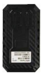
Your tracker has a built-in magnet. Place the tracker in any location that is not surrounded by metal (it can't get a GPS signal when surrounded by metal). Ideally, the tracker is placed facing up toward the sky, however, this is not required.
