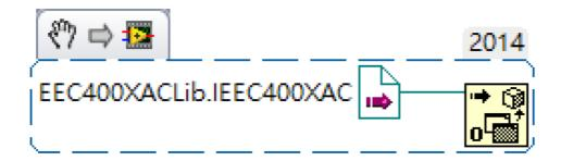
6. Create an Invoke Node function and connect the reference to the output of Automation Refnum and then click on the Method and select Initialize to initialize the connection with device.
