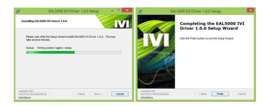
The IVI driver would be installed under the path of "<Program Files>\IVI Foundation\IVI". For the files of the \*.dll file would be located in the "Bin" folder. And the necessary help documents will be in the folder of "..\Drivers\EEC400XAC".
