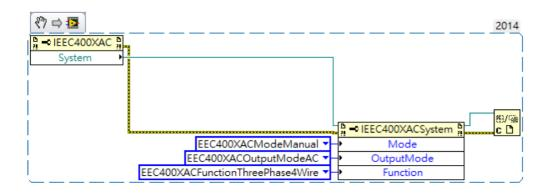
Before we configure the parameters on the EEC400XAC power supply, we have to switch the operation mode. On the 400XAC, it could set to 1phase-2wires, 1phase-3wires and 3phases-4wires. Also, the 400XAC capable of offering AC or DC power source. For the control method, it is capable of switching to Manual mode, Program mode and IEC61000-4-11 procedure.
