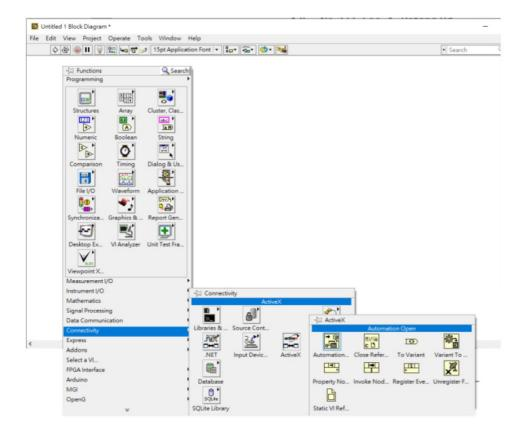
Open the Function Palette by right-clicking on the block diagram. Then select Connectivity -> ActiveX. Select or drop the Automation Open function on the block diagram.
