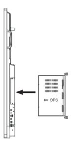
1. Insert the OPS into the slot along the track on both sides.
