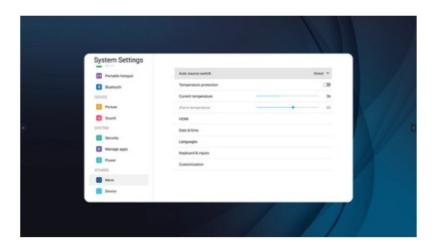
**Note:** When the temperature protection is turned on, if the current temperature exceeds the alarm temperature, countdown is on for the LED turn off. If you want to cancel shutdown can be canceled within 30 seconds.
