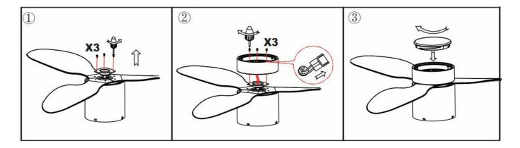
Remove 3 screws from the motor.
