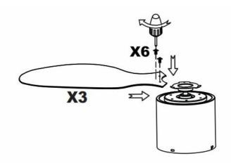
One blade at a time, Align the blade with the 2 holes in the motor, tighten screws securely. Repeat for the remaining 2 blades.
