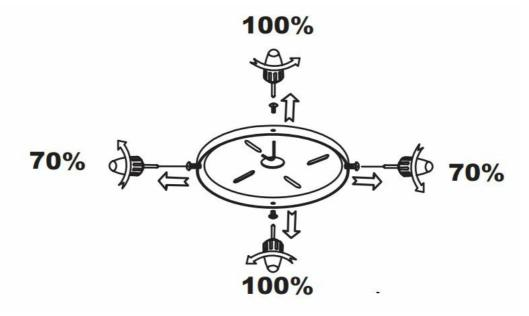
100%(completely) remove 2 screws from the moun?ng plate for later use. 70% remove 2 screws from the moun?ng plate.
