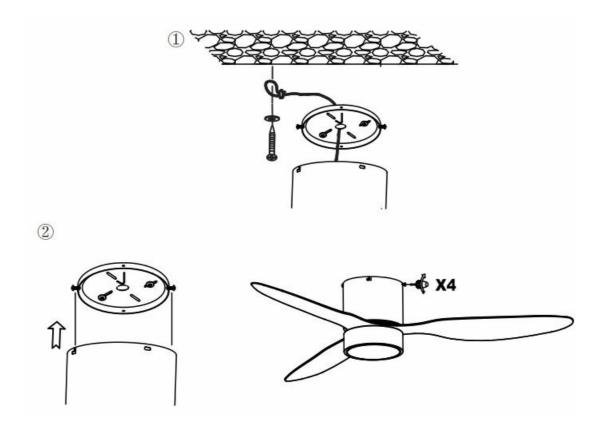
Install the cable to the ceiling with screw and washer provided. Install the whole fan to mounting plate with 4 screws.
