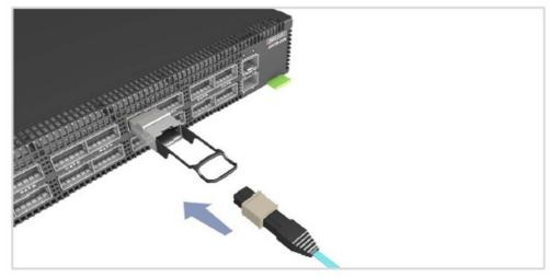
• Note: The upper 16 ports support up to 24 W per port, and the lower 16 ports support up to 14 W per port.
