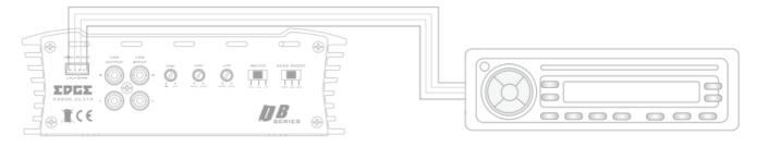
**NOTE** When using high level input it is not necessary to connect the remote turn on wire. Do not connect both high level and low level input at the same time
