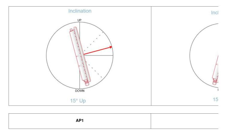
As for calibrating direction, AP will need to also be standing up. However, when adjusting the direction, you will need to slowly move the AP to the right or the left. So basically, if one AP is adjusted 90 degrees to the East, the other AP will need to be adjusted 270 degrees to the West.
