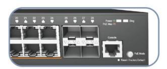
1. Verify basic device operation by checking the system LEDs. When operating normally, the Power and Diag LEDs should be on green.
