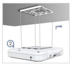
1. At the installation location on the ceiling, use the mounting bracket to mark four holes for the plugs and screws (included in the screw kit).
