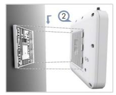
1. At the installation location on the wall, use the mounting bracket to mark four holes for the wall plugs and screws (included in the screw kit).
