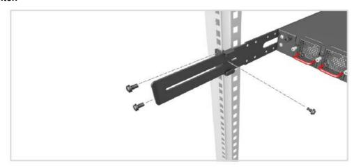
Mount the switch in the rack and secure it with rack screws.
