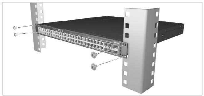
Use the included screws to attach the front- and rear-post brackets.
