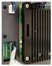
2. Insert the SD card into the corresponding card slot with the contact side facing up, making sure it will not fall out.
