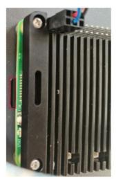
3. Use tweezers to hold the SD card and pull it out.
