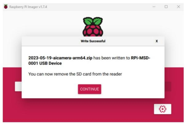
17. Close Raspberry Pi Imager, remove USB cable and power on the device again.
