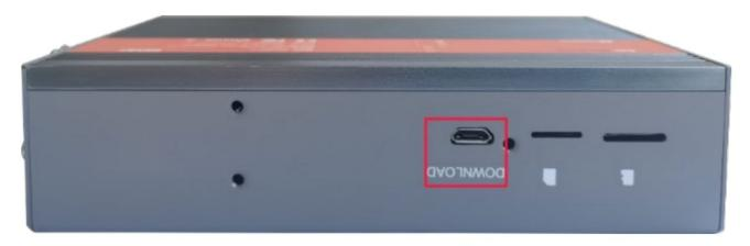
3. Connect the power cord and USB flashing cable, as shown in the figure below.
