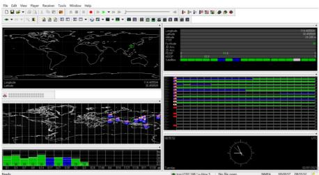
If the Fix Mode is displayed as No Fix, it means that the positioning failed, which is usually caused by the antenna being indoors. Please put the module or antenna outdoors for testing.
