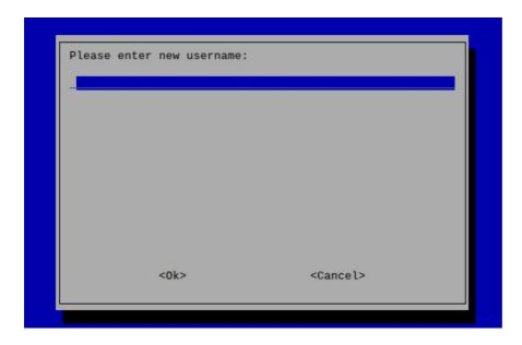
Then set the password corresponding to the user according to the prompt, and enter the password again for confirmation. At this point, you can log in with the user name and password you just set.
