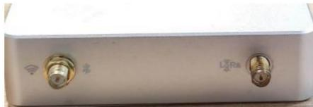
According to the icon next to the antenna, install WIFI/BT antenna on the left and LoRa antenna on the right. A paper logo is also attached to the antenna.
