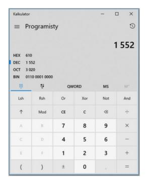
**EMU CLASSIC** receives temperatures from the EGT to CAN device on ID 1552 and 1553 (610h and 611h). **EMU BLACK** receives temperatures from the EGT to CAN device on ID 1632 and 1633 (660h and 661h).
