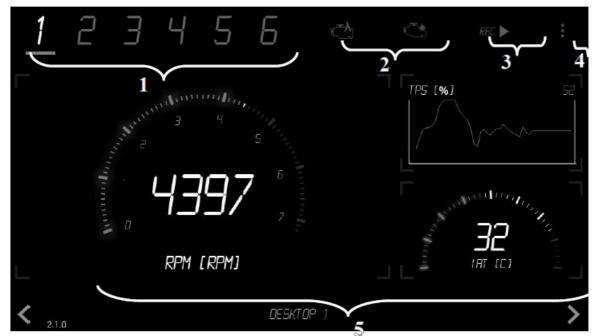
Option menu (4) allows to change display color (blue, amber), display mode (three or six channels on desktop), units( metric, imperial).
