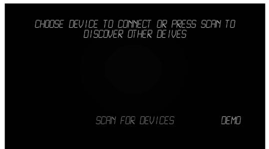
After several seconds a list of found Bluetooth devices will appear. Choose EMUBT device. If EMUBT device will not appear on the list, check connection between EMU ECU and Bluetooth module and LED status.
