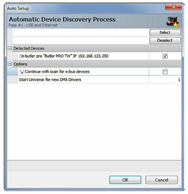
• Using this device setup dialog you can set the DMX universes as well as the required RDM feedbacks for the channels of the Butler PRO When finished close the device setup dialog with Ok.
