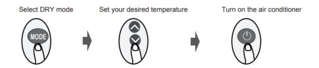
**NOTE:** In DRY mode, fan speed can not be set since it has already been automatically controlled. **FAN Mode**
