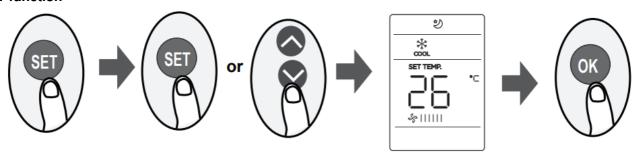
Press the SET button to enter the function setting, then press SET button or TEMP or TEMP button to select the desired function. The selected symbol will flash on the display area, press the OK button to confirm.
