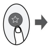
Push this button when remote controller is on, the system will automatically revert back to the previous settings including operating mode, setting temperature, fan speed level and sleep feature (if activated).
