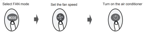
$\label{eq:NOTE:} \textbf{NOTE:} \ \textbf{In FAN mode, you can't set the temperature. As a result , no temperature displays in remote screen.} \\ \textbf{Setting the TIMER}$
