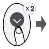
The unit will operate at high fan speed (while compressor on) with temperature automatically set to 8 C/46 F. **Note:** This function is for heat pump air conditioner only.
