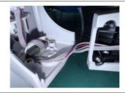
The rain bucket can now be completely separated from the main unit.
