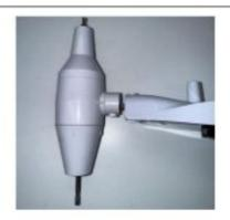
There is a fixing screw between the wind speed and wind direction sensors. Loosen this screw.
