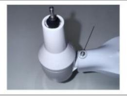
Remove the screw, and the wind speed and direction sensor will separate from the main unit.
