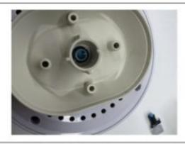
4. To replace the temperature and humidity sensor, simply follow the above steps in reverse order: first insert the new sensor module, then install the four rain shields, and finally tighten the screws.
