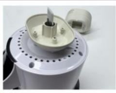
Unplug the temperature and humidity sensor module and replace it with a new one.
