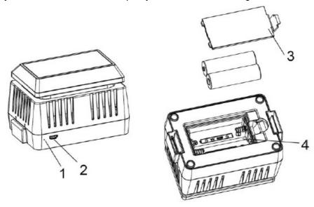
2. Insert two AA batteries and close the batterydoor.
