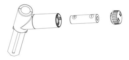
Place one AA alkaline battery in the sensor and close the battery door.
