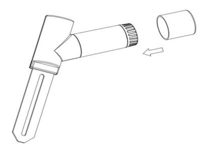
Place the extra protection sensor cap over the battery door to achieve better sealing against moisture.
