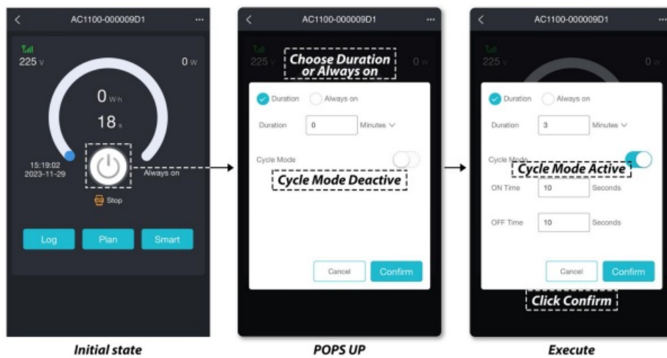
Figure 6 Manual Mode program Illustration
