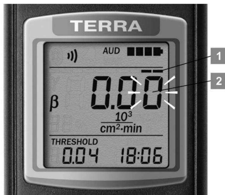
Figure 18 – LCD of the dosimeter (the submode of alarm threshold level programming)
