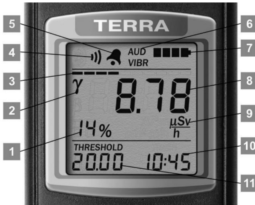
Figure 3 – LCD of the dosimeter (the mode of photon-ionizing radiation DER measurement)
