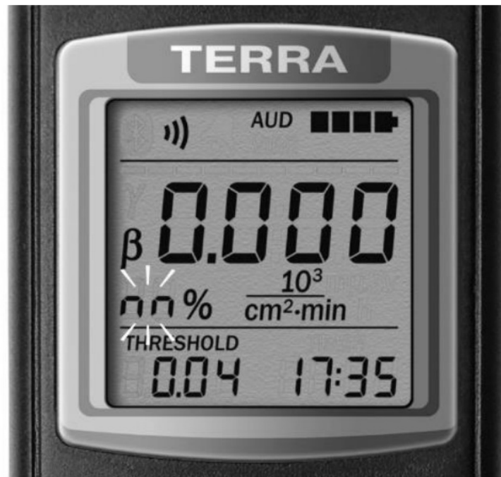
Figure 17 – LCD of the dosimeter (measurement restart)
