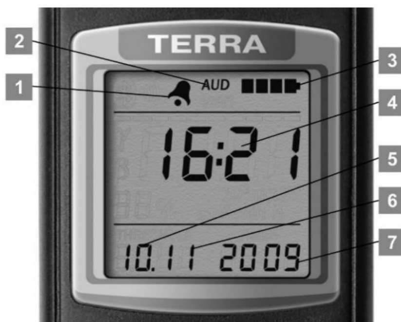
Figure 21 – LCD of the dosimeter (the clock mode)
