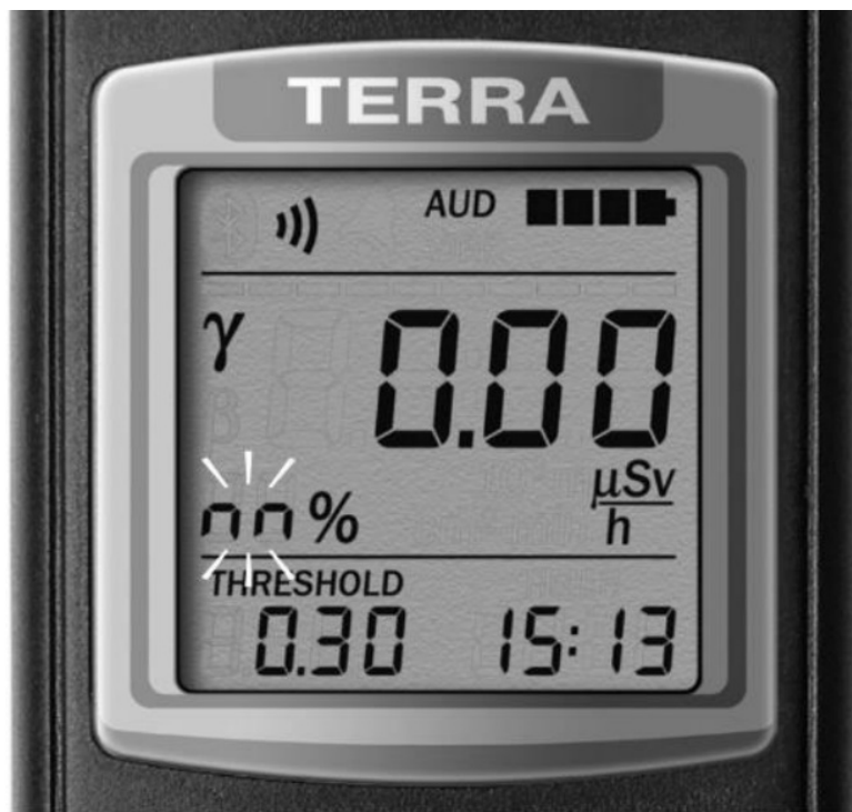
Figure 6 – LCD of the dosimeter (measurement restart)
