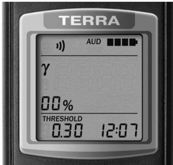
Figure 4 – LCD of the dosimeter (viewing the value of specified statistical error)
