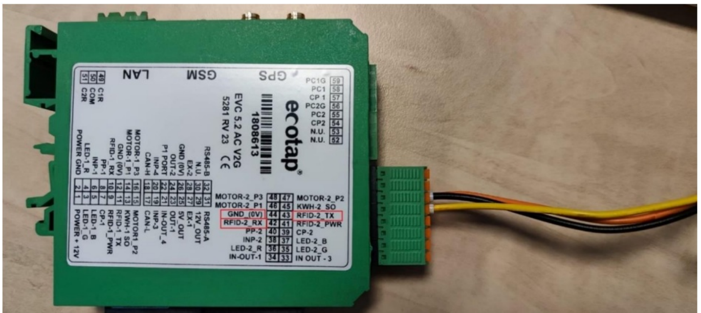
Figure 5.4 – Connecting the USB to TTL cable to the controller (EVC 4.x).
