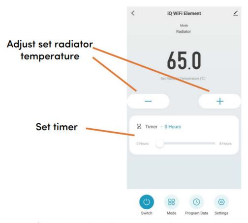
Figure 11 | Radiator mode interface on Smart Life app
