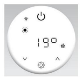
The temperature displayed is the set temperature. Set temperature range is 7-30 °C and can be adjusted using the \(^{\text{A}}\) and \(^{\text{V}}\) buttons. You can check the current room temperature when you are connected to the app. The temperature set in comfort mode also applies to comfort intervals when they occur in program mode.
