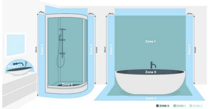
Figure 1 | Bathroom installation zones
