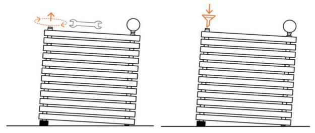
Figure 5 | Removing radiator cap and using funnel to fill
