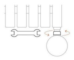
Figure 4 | Tighten element at main nut
