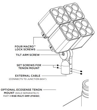
F170 QUAD can also mount to any 2-3/8" OD pipe or tenon.
