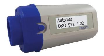
The read-out head ecom-AK enables the recall of data made available by digital firings automats. Information like trouble sources, error history, flame signal and operation voltage are received by the ecom-AK as optical signal at the reset button of the firing automat and shown on the graphic display.
