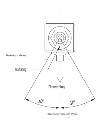
• Diagram of sensor fitted in a pipe:
