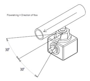
• Loctite 577 is used at the factory to seal the thread, but packing yarn/packing tape can also be used.
