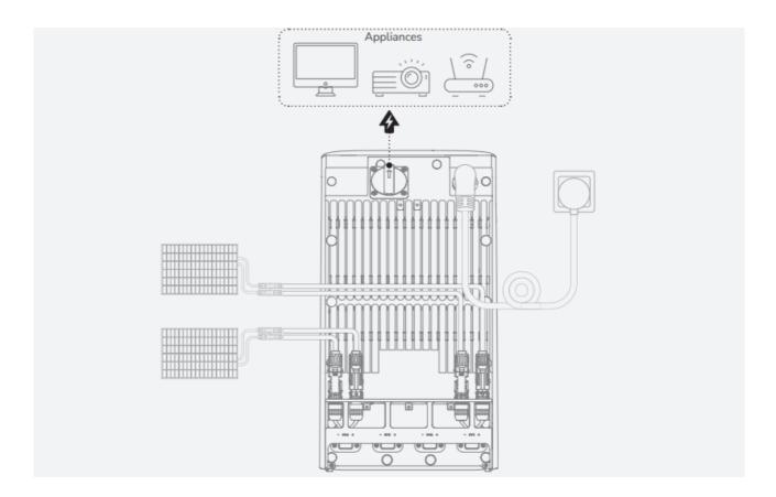
Option 2: Connect to a microinverter to add power input
