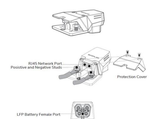
This adapter comes with two RJ45 CAN Bus ports, each port can be connected to EcoFlow Power Kit Console or another adapter. When two or more battery packs are connected and the RJ45 CAN Bus port is not connected to either of the above modules, an RJ45 CAN bus terminator MUST be connected to the port to ensure proper communication throughout the system.
