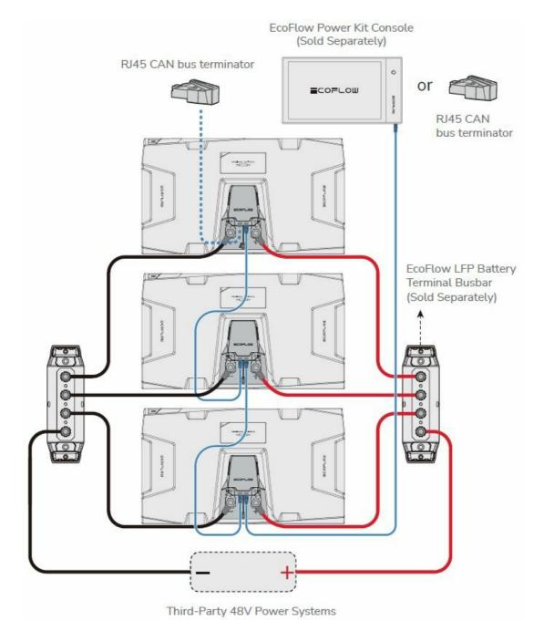
The user should select the appropriate connection cable according to the power of the third-party power system and the discharge current of the battery.
