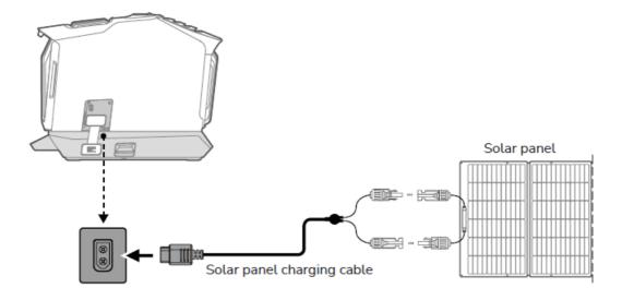
It is recommended to power off Wave 2 when charging the battery pack for higher charging efficiency.
