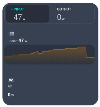
The Input tab displays the unit's overall input power and the details of each input port, including the input power of solar energy, car charging, and AC power supply. When solar energy or car charging is used, you can view the change of the power curve in real-time. If DELTA Max or DELTA Pro is connected, you can also view the status of the extra battery pack.
