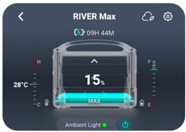
The battery temperature is displayed to the left of the unit image, where H represents hot temperatures and C represents cold temperatures. The remaining battery level is displayed to the right of the unit image, where F represents a 100% level and E represents a 0% level.
