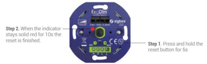
Please Note: All configuration will be reset after the device is reset or removed from the network.
