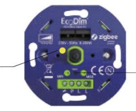
**Step 2**. Press the reset button for 5 times.
