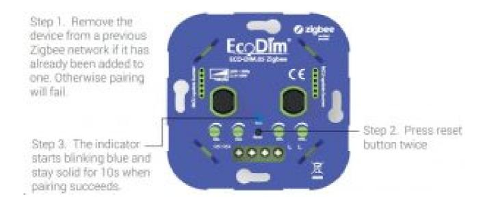
3. REMOVE: There are two methods to remove the device from the Zigbee network.
