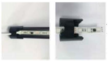
4. Screw the base into the lamp body
