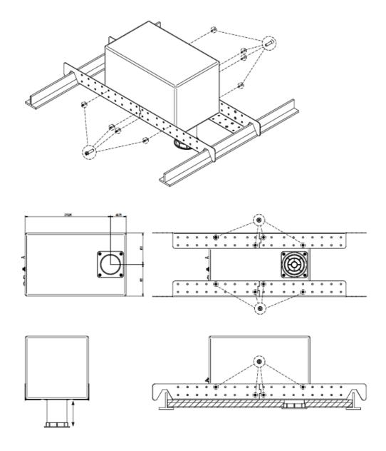
Diagram for suspended ceiling installation.
