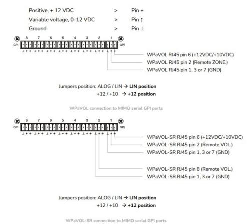
Connecting cables can be up to 500 meters with a minimum section of 0.5 mm.
