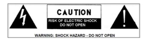
The lightning flash with the arrowhead symbol, within an equilateral triangle, is intended to alert the user to the presence of uninsulated "dangerous voltage" within the product's enclosure that may be of sufficient magnitude to constitute a risk of electric shock to persons.
