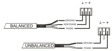
Live or direct signal > Terminal + Cold or inverted signal > Terminal - Ground > Terminal  $\perp$  For UNbalanced connections, leave the terminal - unconnected.
