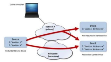
**Note:** in this mode, if (by mistake) the primary and secondary ports connect to the same Ethernet network, Dante Controller will no longer have access to the network configuration control and routing Dante™ of the MIMO7272DN ports. This control is recovered when one of them is disconnected from the same network as the other.
