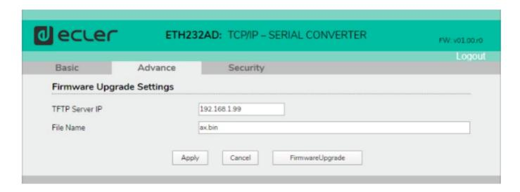
The advanced settings allow to execute the firmware upgrade of the device using a TFTP server utility installed on your PC.
