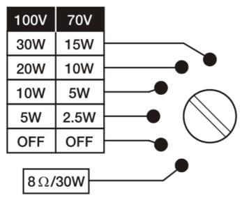
Figure 1: rear panel's power selector
