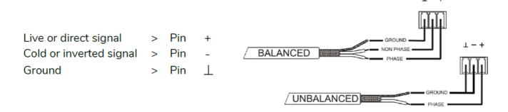
For unbalanced connection short-circuit pin  $\perp$  to pin – as reported on the picture.
