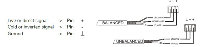
For unbalanced connection short-circuit pin  $\perp$  to pin – as reported on the picture.
