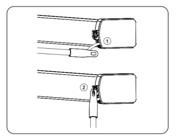
**Note:** On Sheer Shadings ordered with Power and on the right side, the cable may be wrapped around the hook. This is normal. You may unwrap, if you desire, as this does not affect functionality. You still need to connect the cable into the motor head.
