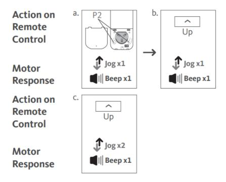
If the motor has no response, it already has a Maximum or Minimum speed.
