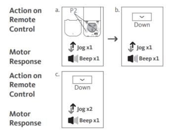
If the motor has no response, it already has a Maximum or Minimum speed.
