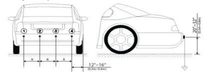
**Sensor Install:** Sensors must be installed in order 1-4 from left to right with control module harness entering trunk near sensor #4. If only using 2 sensors for the install, it is recommended to use sensors 2 and 3.
