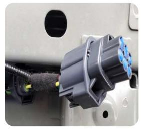
Vehicle that is equipped with trailer tow wiring
