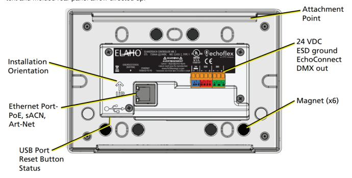
2. Install the prepared five position screw terminal connector (24 VDC, ESD Ground, and Echo Connect control wires) and the utilized three-position connector (DMX) to the designated receptacle(s) on the rear panel of the unit. This instruction assumes you have prepared the cables and terminated them according to the provided instructions for your installation type.
