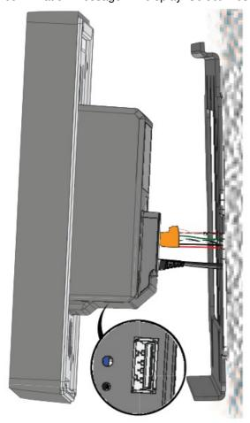
**CAUTION:** The update process may take a few minutes. Do not shutdown or remove power from the touchscreen until the update process has finished. When prompted, restart the touchscreen by pressing the Reset button located near the USB port.
