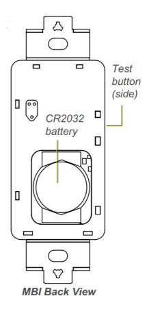
Use hand tools when installing. Over-torqueing with a power tool can damage the switch. Three different mounting options are available:
