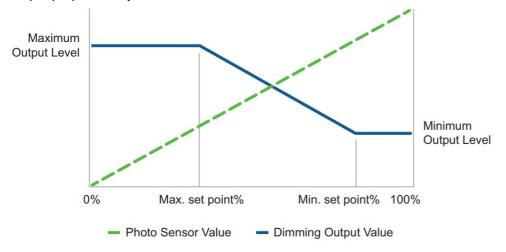
The rate that dimming output changes is defined by the parameter open loop dimming rate which defines the time for dimming to go from 0% to 100% or vice versa (default 65 seconds).
