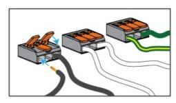
Terminate EchoConnect wiring using provided WAGO connectors.
